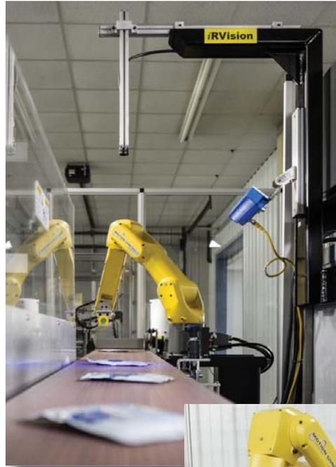
*Advances in vision sensor technology has led to the development of a variety of end-of-arm tooling that has evolved into more nimble product handling for case packing.*
