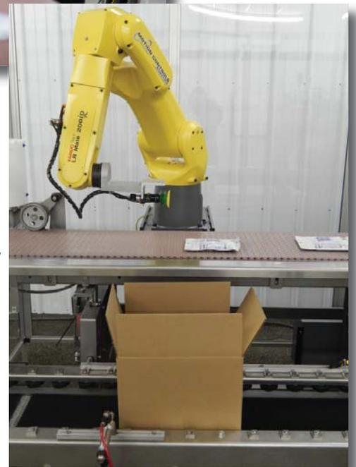
*Combi's robotic Ergopack® provides the flexibility of parking the robot while hand packing small runs of product*
