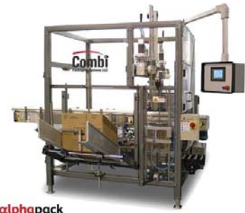
Top loading Servo Pick and Place Packers featuring multi-axis servos for precise and safe placement of products into erected cases
