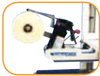
Tip up top tape head simplifies roll replacement
