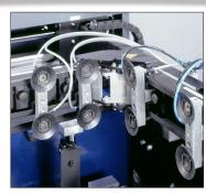
Unique hinged pickup and folding frame reliably opens cases by placing erecting frame suction cups on two panels of blanks
