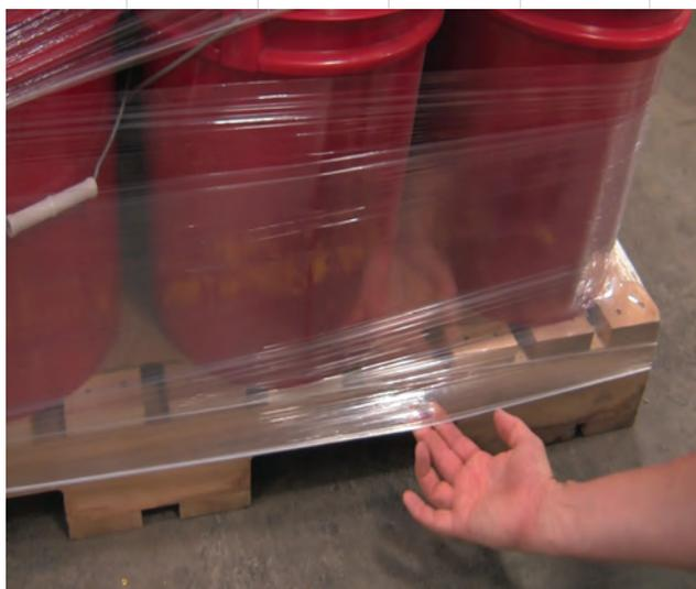
Pallet Grip places the film cable around the shipping pallet and locks the load to it.
