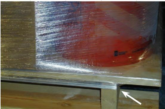
The rolled up film cable is driven down on the pallet to about an inch and a half below the topboards, where it can't be damaged by fork truck entry.
