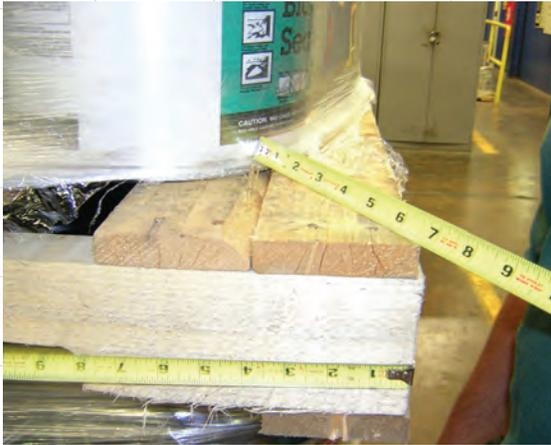
Product is inboard and not "locked" to the pallet with stretch film. The film is wrapped around the product only, creating the opportunity for the load to slide off the pallet.
