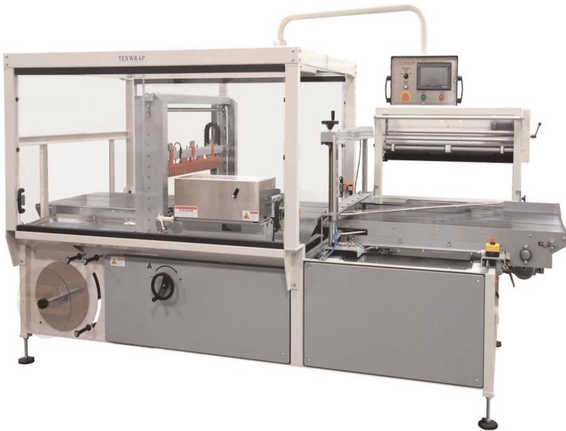
The 2410 is Texwrap's intermittent motion side seal machine designed to run large products at moderate speed. A new version of the 2602, it has a capacity of 24" wide and 10" tall. The 2410 is versatile enough to accommodate a variety of product sizes and configurations.
